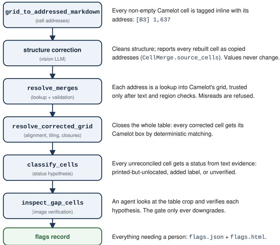
Figure 1 — The provenance pipeline. Grounding is deterministic. The two LLM agents, correction and inspection, only report and verify.
